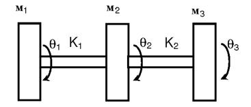
47. Calculate approximate natural frequency of a system by using Holzer's method?
